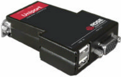
Figure 1. Uniport (Direct connect)
