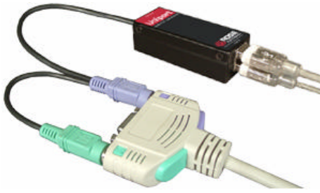
Figure 5, Uniport to a KVM cable
