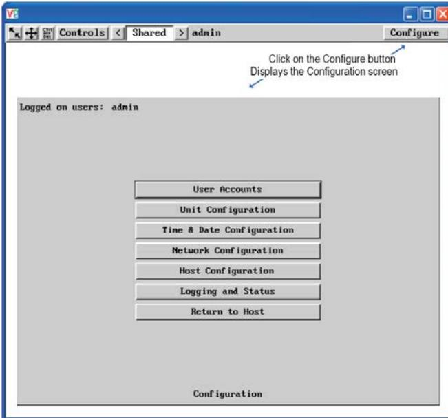
The configuration menu allows you to set-up user accounts, configure the unit, set the time and date used to time stamp the log file, configure the network, and view the logging and status.
