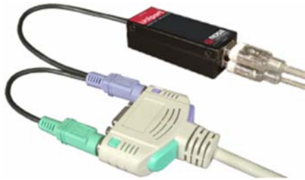
Figure 5, Uniport to a KVM cable
