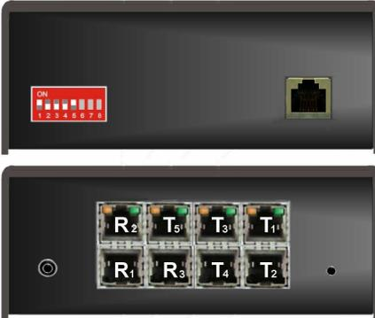
The 5 x 3 configuration allows you to connect 5 computers to the Orion LC and display the video (+audio option) on up to 3 DVI monitors.
