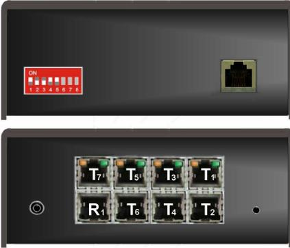
The 7 x 1 configuration allows you to connect 7 computers to the Orion LC and display the selected computer's video (+audio option) on 1 DVI monitors.
