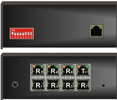
The 1 x 7 configuration allows you to connect 1 computer to the Orion LC and display the video (+audio option) on up to 7 DVI monitors.
