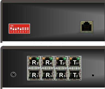
The 3 x 5 configuration allows you to connect 3 computers to the Orion LC and display the video (+audio option) on up to 5 DVI monitors.
