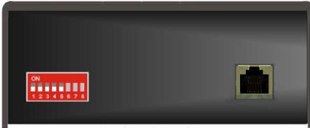
Set the dip switches so that switch 1, 2, 3, 4, and 5 are all in the “OFF” position.
