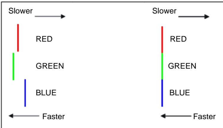
Figure 4. Color skew delay compensation
