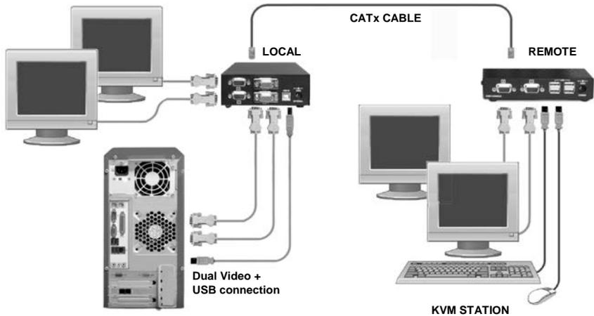
Figure 3. Dual Video Connections
