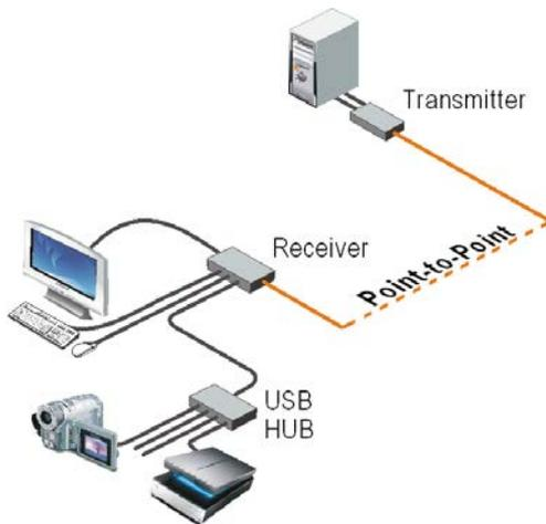
**Figure 2. Typical Installation**
