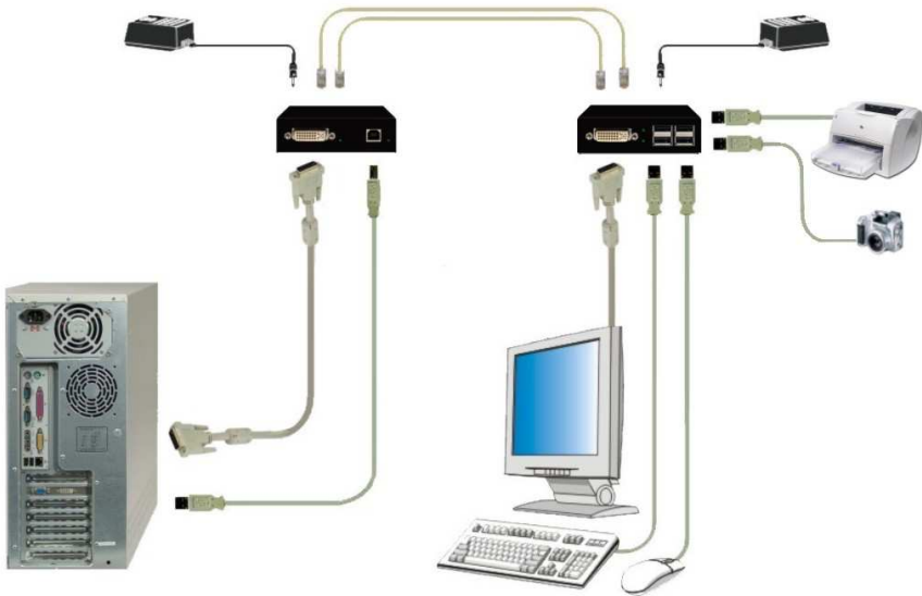
Figure 7. Single head Installation (USB-2.0)
