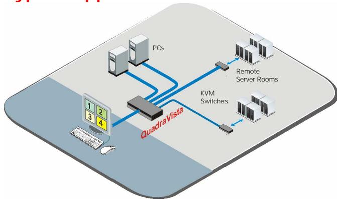
**Models** The QuadraVista Quad Video KVM Switch is available in a single user, four computer model. Adding KVM switches to it can expand the system to 1,000s of computers and serial devices.
