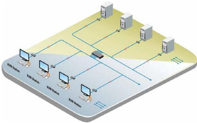
**Overview** The Orion XC system consists of the main unit, a transmitter unit for each connected computer and a receiver unit for each connected KVM workstation. The transmitter and receiver units are available in several models. These models are selected to match the computer's and KVM workstation's configuration. The transmitter and receiver units are connected to the Orion XC using CATx cable.
